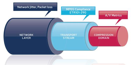
Iris analysis goes beyond the network and transport stream layers to allow users to monitor metrics within the compressed domain.
