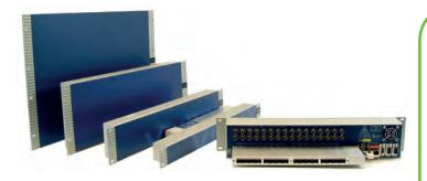
The Sublime optical is a mixed optical/electrical compact router solution ranging from 16x16 in 1RU to 128x128 in 8RU. The optical extension ports are built up as modules of 16 in +16 out, and ranges upto 128 in+128 out.
