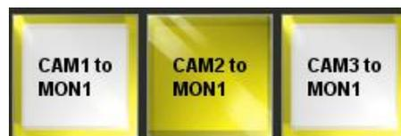
Source-to-destination buttons are typically used in single bus panels.
